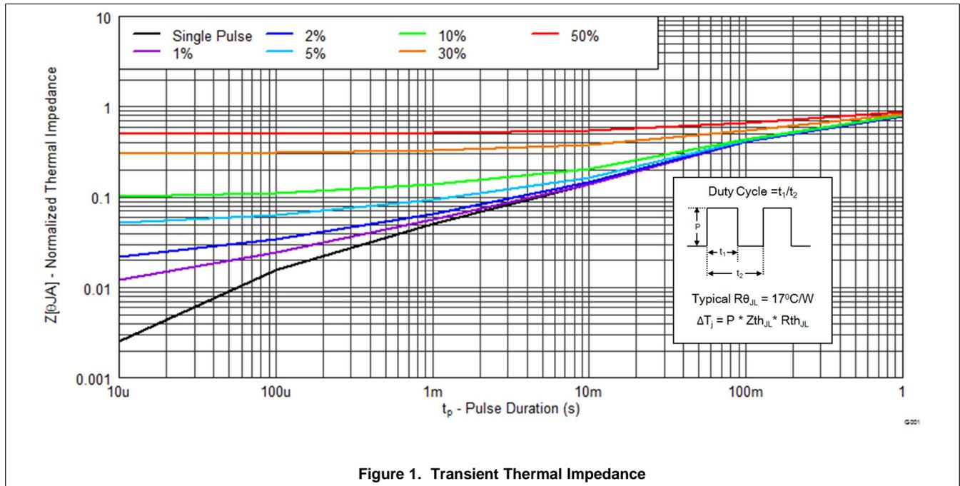
Figure 1. Transient Thermal Impedance
