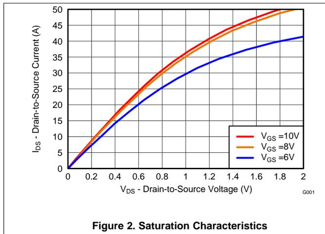
Figure 2. Saturation Characteristics
